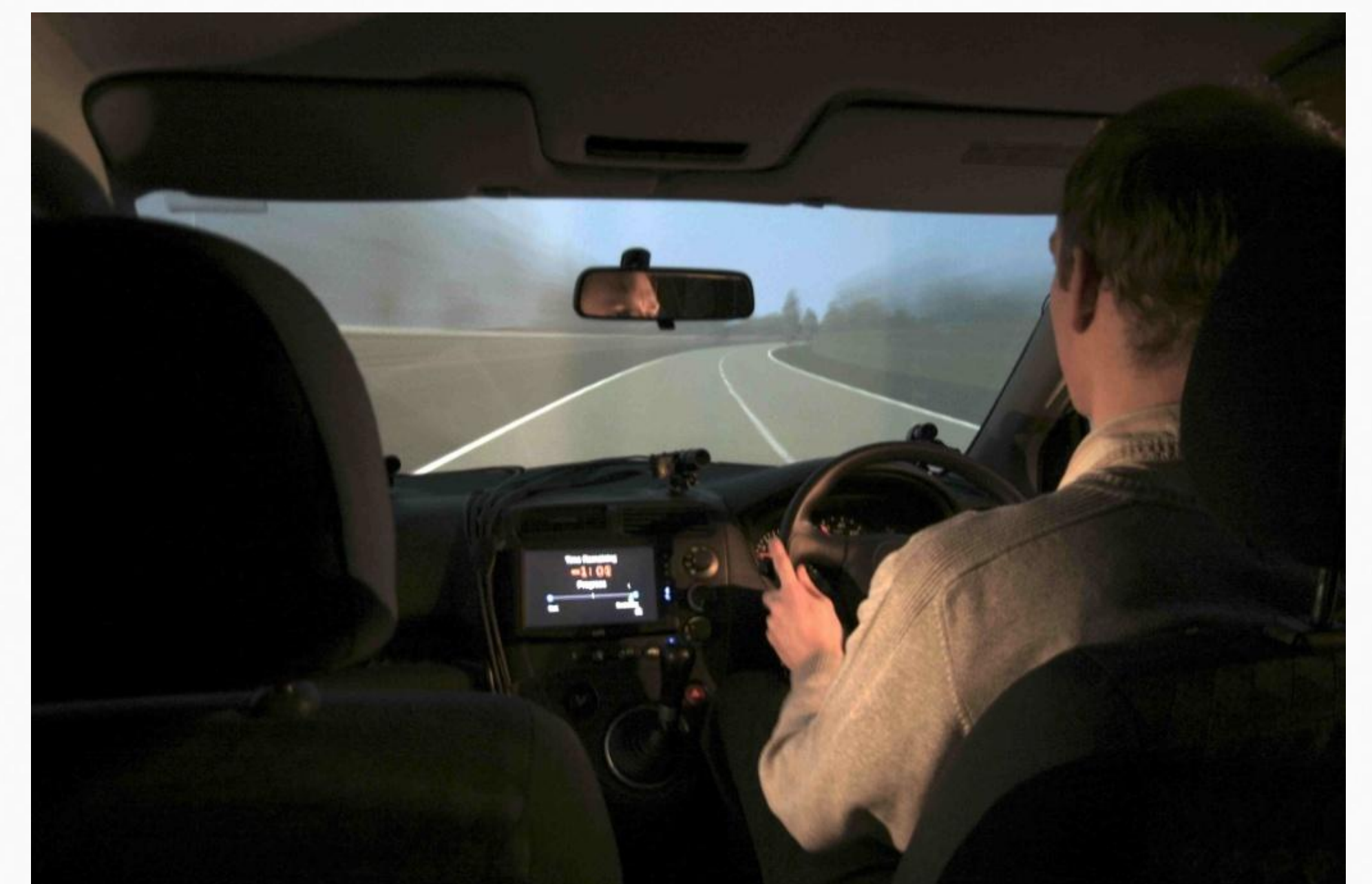
Driving simulation to measure perception of differences in vehicle performance: in naturalistic driving and in specific controlled action sequences
