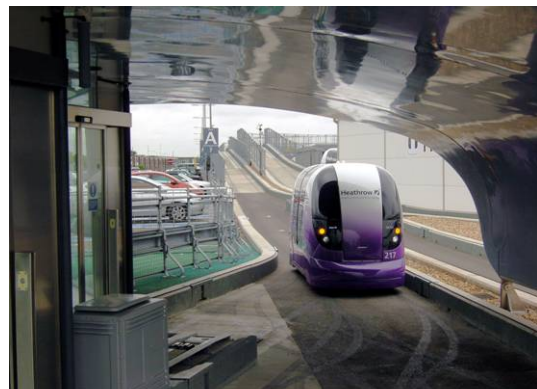
A Heathrow PRT 'pod' descending from the elevated guideway to a car park station
